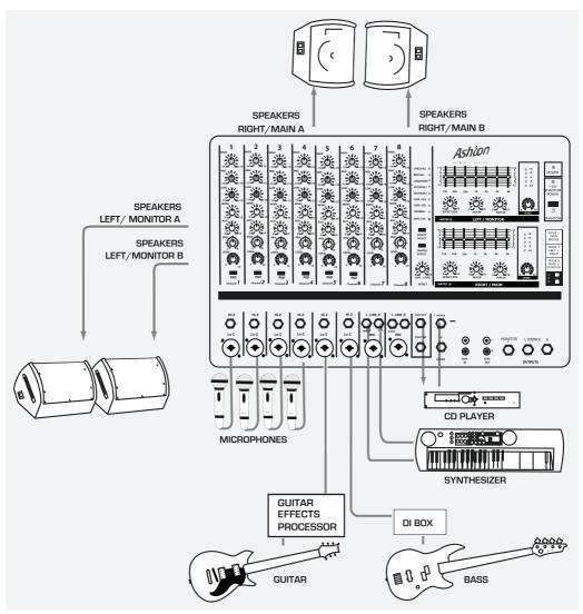
This setup is perfect for a band rehearsal or live setup. To setup, simply follow the diagram above with the relevant instruments/devices/speakers.
